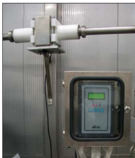
TOR-AL METAL DETECTOR WITH WATERPROOF COMP-AL CONTROL BOARD FOR MEAT SAUCES INSPECTION
