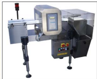
TUNN-AL METAL DETECTOR ON STAINLESS STEEL STRUCTURE FOR FISH PACKINGS INSPECTION
